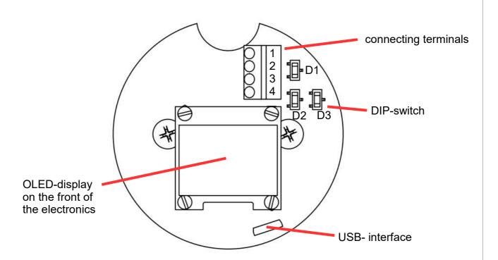
The electronics can be configured via the USB interface. The operating instructions and the software can be found on our homepage for the respective device.
