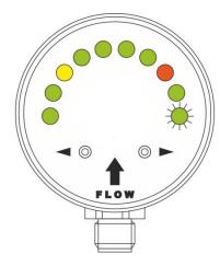
last LED flashing = the flow is above the monitoring range
