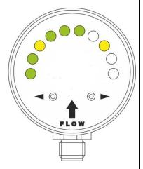
the flow velocity is within the adjusted monitoring range
