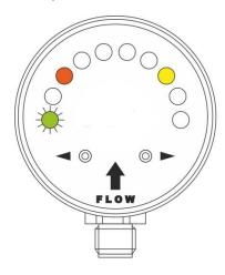
first LED flashing = the flow is below the monitor monitoring range
