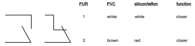
switching contact temperature opener / level switch closer or opener
